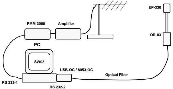
Fig. 2-1 Typical configuration to test irradiation immunity
